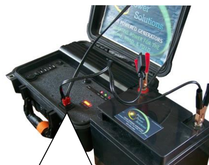
Image shows 44Ah AUX battery & MPI cable connected to a 201 kit multiport with a 45W panel also connected to the Solar In (panel not in frame).
